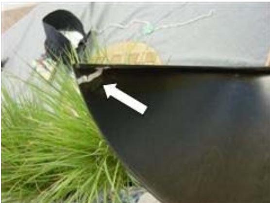
Larry explained that cutting out a portion of the gauge panel cover flange at the left end will allow easy removal of the cover. Here is the finished cover:
