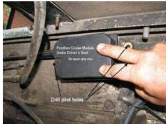
John positioned the cruise control module under the driver's seat floor on the upper step riser.
