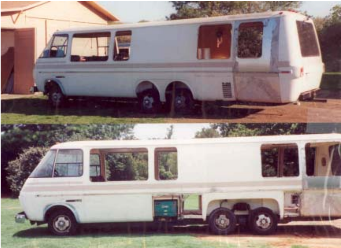
6. Slid rear bogie assembly rearward 20 inches.
