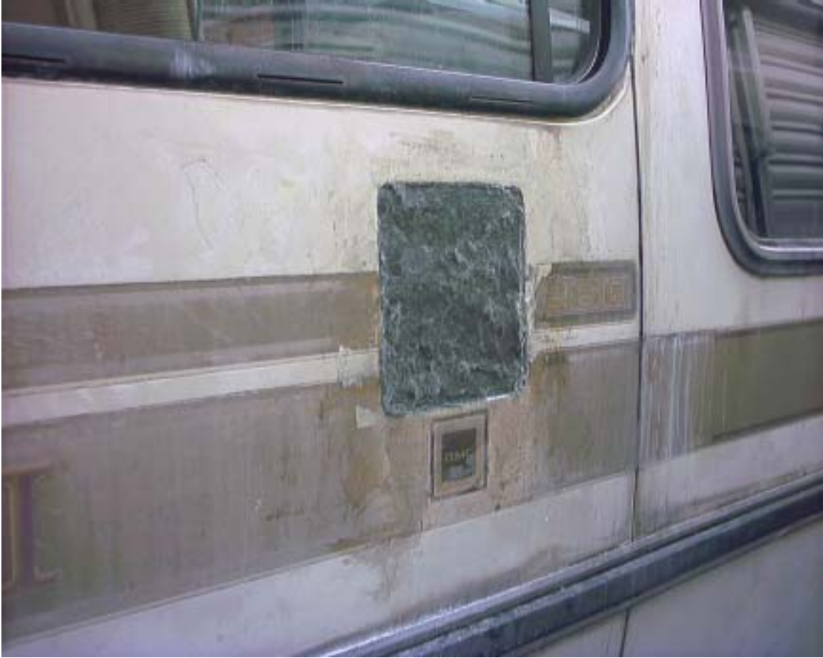
The “Dyna-Hair” forms a strong patch due to the fiberglass fibers suspended in the resin.
